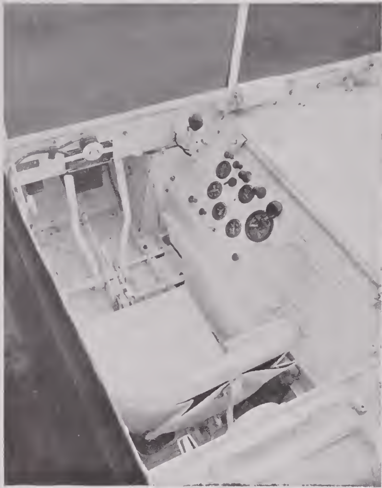
FIGURE 54. Instrument board and controls in driver's compartment of M-29C Weasel.
